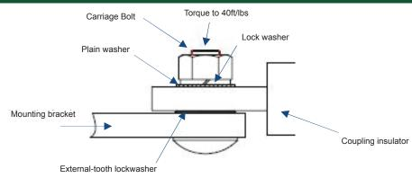
**Step 1:** Once Mounting Bracket is attached to the Cross Arm the Carriage Bolt is installed from bottom of mounting bracket
